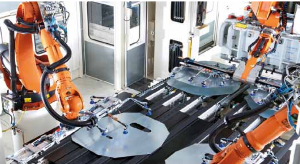
Centering station with vision system for part orientation
