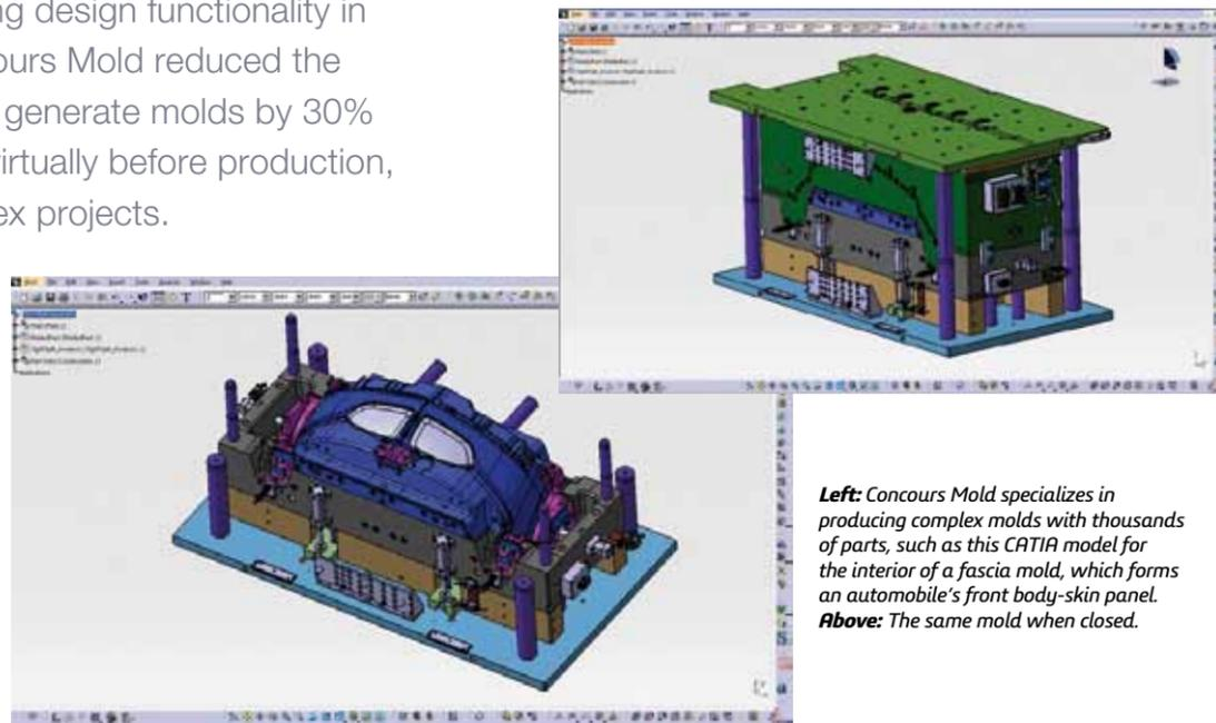
**Left:** Concours Mold specializes in producing complex molds with thousands of parts, such as this CATIA model for the interior of a fascia mold, which forms an automobile's front body-skin panel. **Above:** The same mold when closed.
