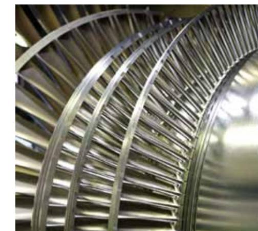
Detail of a low-pressure steam turbine rotor
