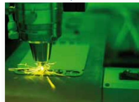
Ceres Fuel cell laser welding
