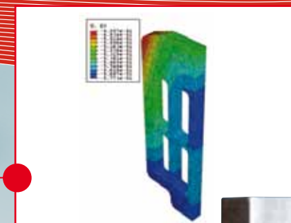
Stack Endplate deflection during assembly
