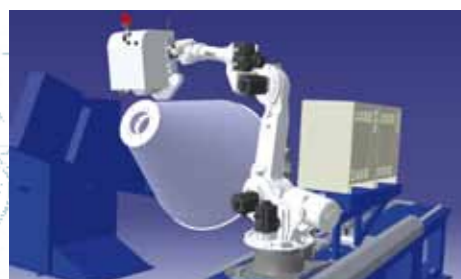
Virtual representation of robot inspection in DELMIA
