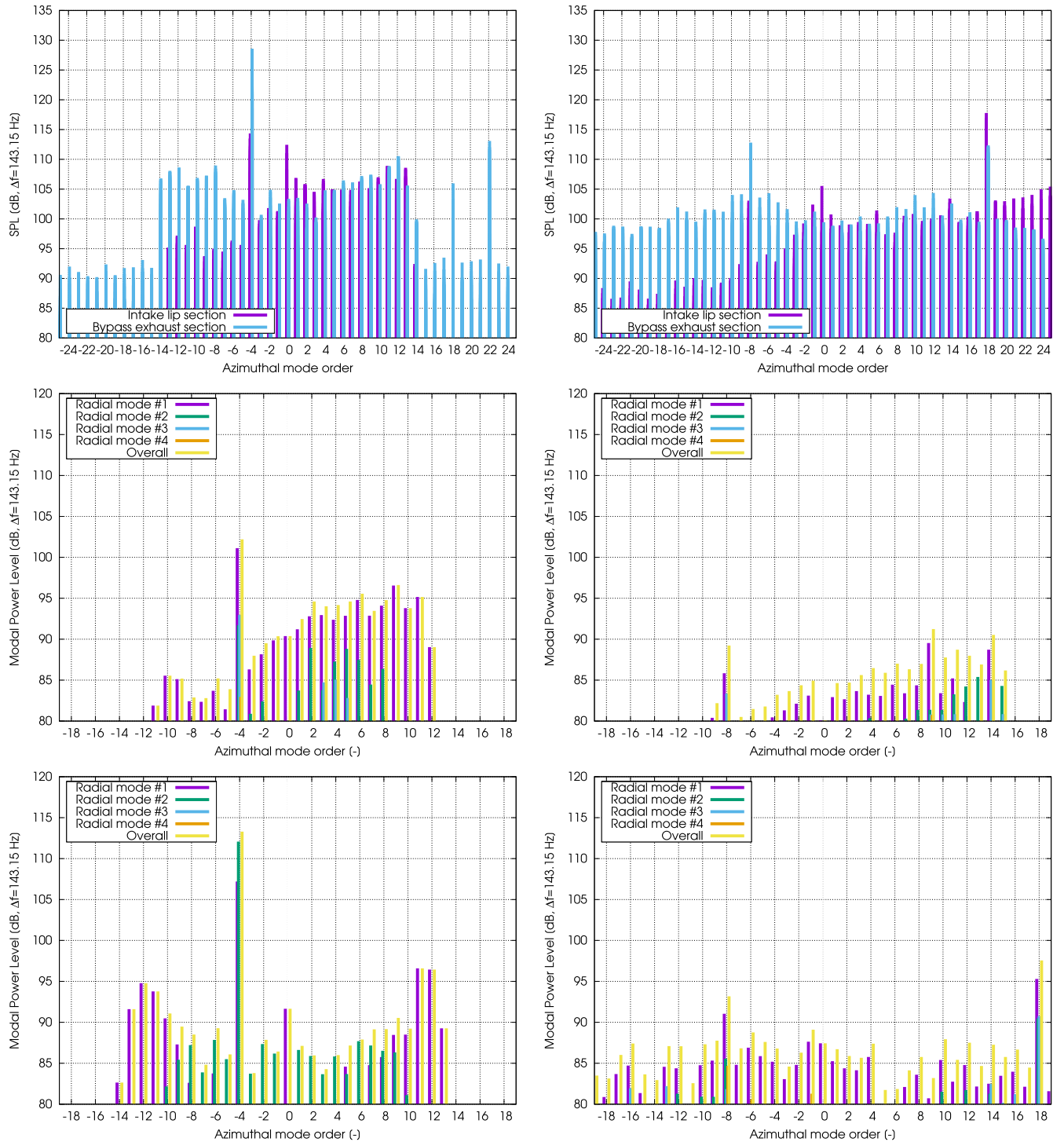
Fig. 21 Circumferential Fourier mode decomposition (top) and cut-on duct modes fitting at the intake lip section (middle) and bypass exhaust section (bottom) for low-noise configuration. 1BPF (left) and 2BPF (right) results.
