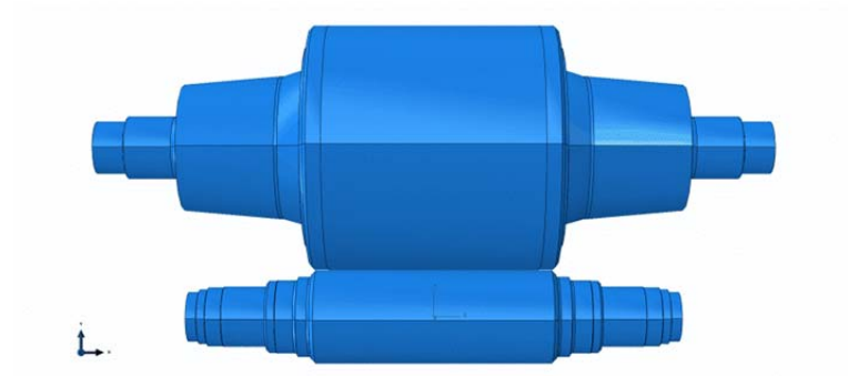
Figure 2. Vertical symmetry applied in a 4 high mill.
