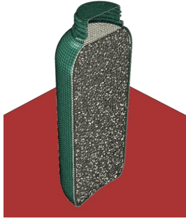
Figure 9. Cross-section view of the drop test simulation model (bottle in green, water in gray, and floor in red).
