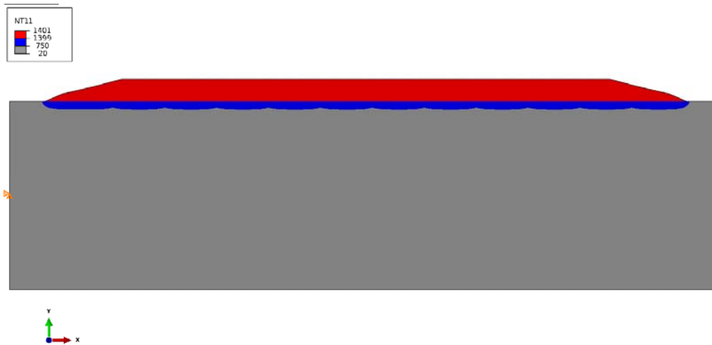
Type 308 L Stainless Steel 80 mm Clad Plate Model
