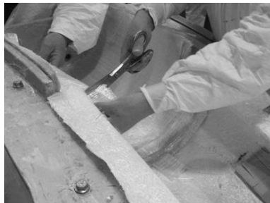
Figure 9. Hand layup of fabric plies in the mold of a wind turbine blade.
