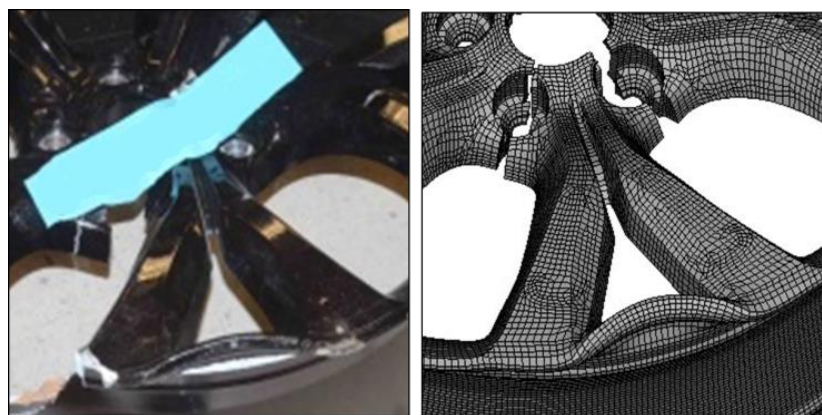
Figure 17. 19" Wheel Damage: Comparison between Lab test and CAE results for spoke loading
