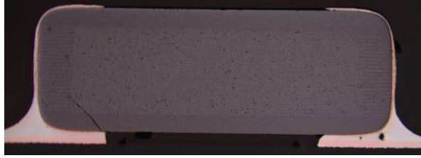
Fig 12. Partial flex crack revealed through cross-sectioning
