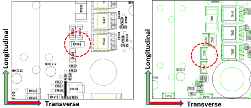
Fig 11. New layout decided based on the simulation results (old layout is included for reference)
