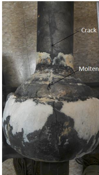
Figure 1. A molybdenum single piece glass melting electrode (GME) with a molten section and a crack extending along the vertical direction of the electrode.
