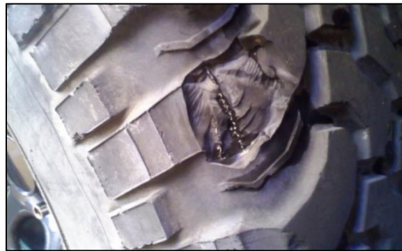
Figure 2 – Depiction of a thermal blowout in a tire tread
