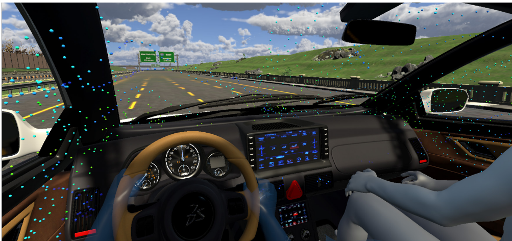
Airflow visualization inside a vehicle. When visualized immersively, the airflow surrounds the user.
