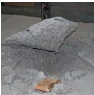
Figure 3. Anchor tensile test with concrete breakout cone
