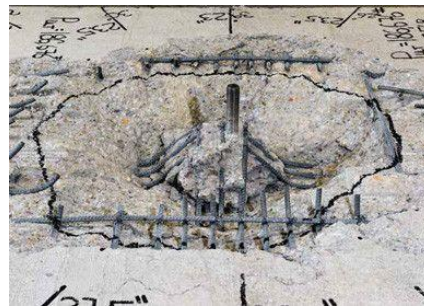
Figure 4. Podium anchorage with local reinforcement
