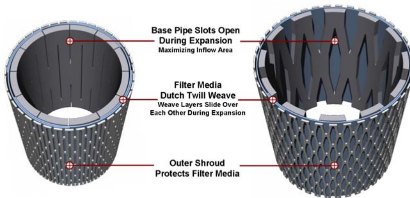
Figure 1 Details of the construction of the ESS
