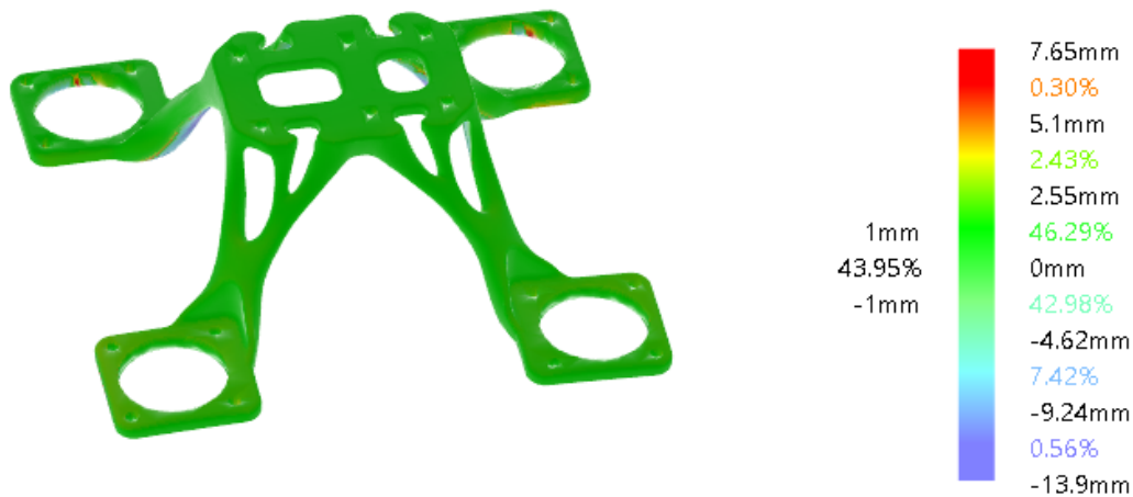
Fig. 7 Deviation Analysis of simulation results w.r.t experimental results
