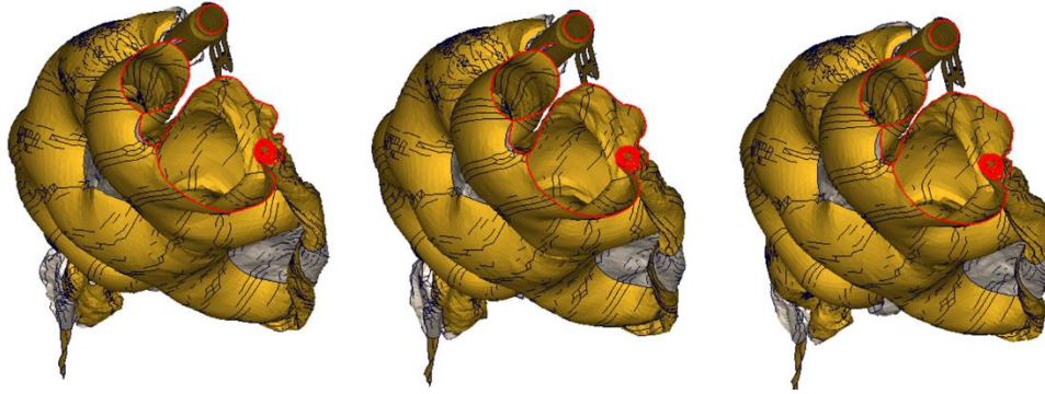
Figure 4. Same position as in Figure 3 with different contact thickness settings for the surface elements (5mm, 3mm, 2mm) for 5mm CEL element size. (Horz 2015)
