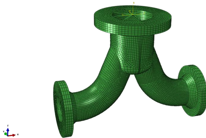
Figure 2: Solid CAD Model of Wye
