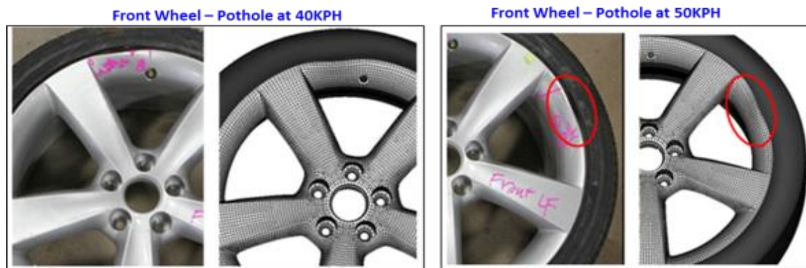
Figure 16. Comparison of Distorted location in Wheel: Test Vs CAE
