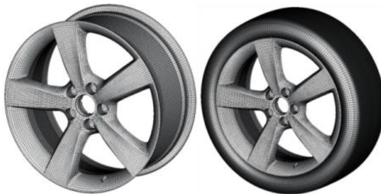
Figure 4. Finite Element Model of Wheel and Tire
