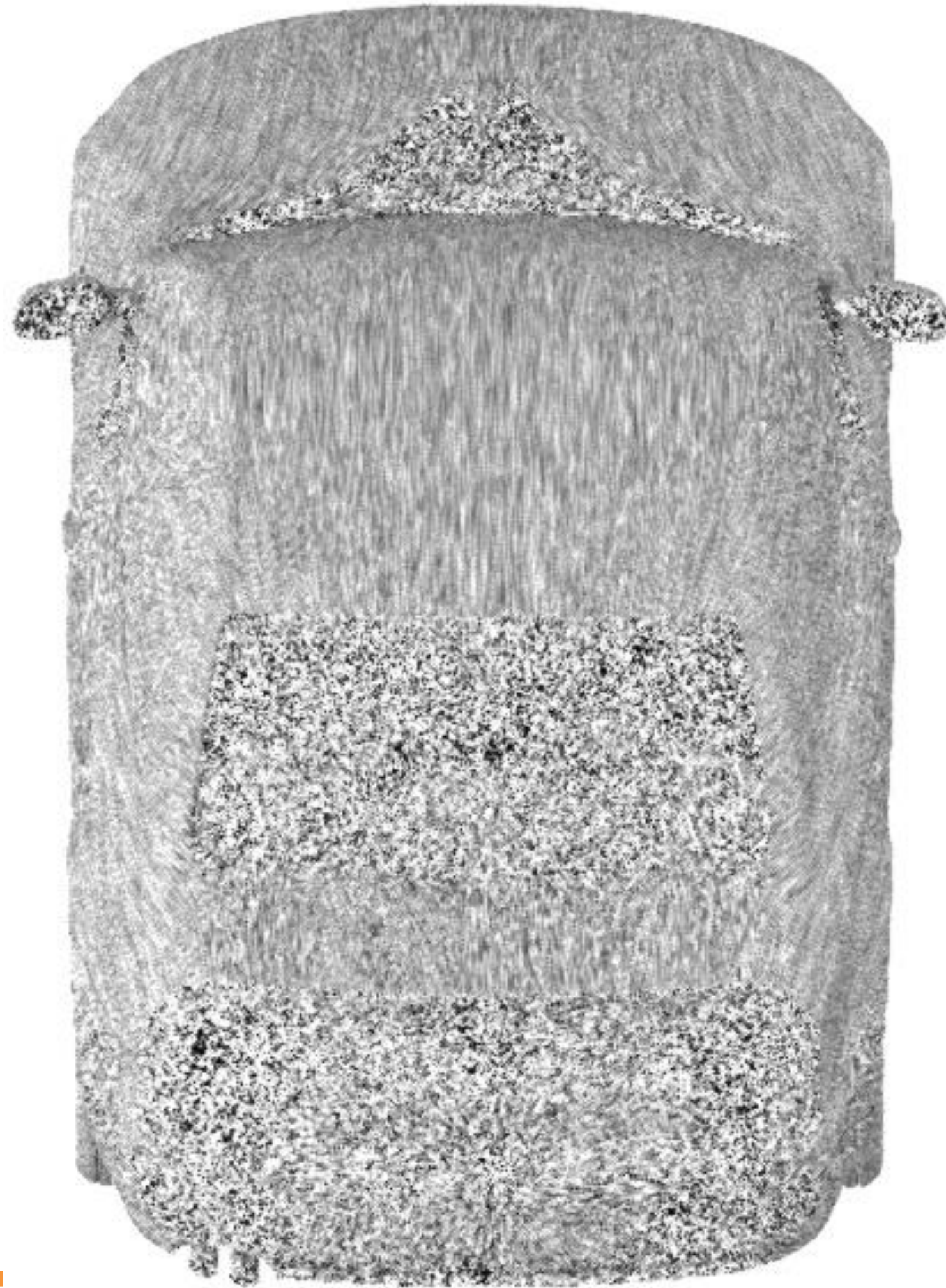
Detached flow NotchBack C_x=0.2808
