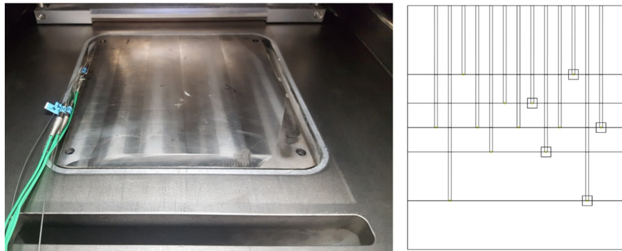
Fig. 14. Image of the thermocouple substrate (left) and an illustration (right) showing the location of the blind holes for thermocouple placement.
