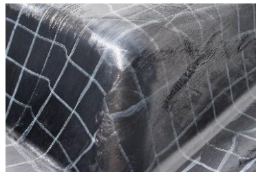
In-plane undulation and gapping
