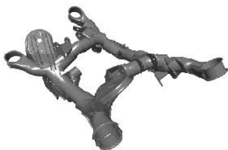
Exaggerated Bending Mode of Rear Subframe
