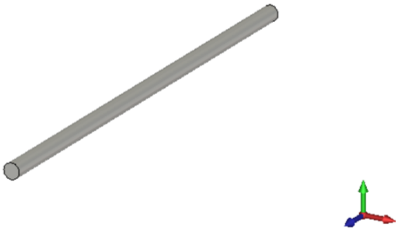
Figure 9: PEC cylinder to be used as the metallic part of the dipole antenna
