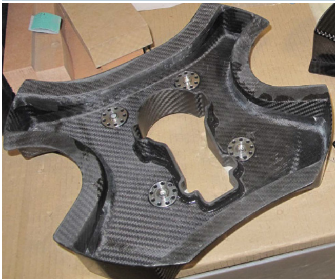
(Top) Final drawings for the Batman winch-gear support plate design. Note phalanges along outer edges (upper right image) that provide additional stiffness. (Bottom) A finished Batman composites component.
