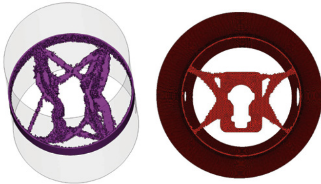
(Left) iXent's first Tosca iteration of the sailboat gear support and (Right) the final output.
