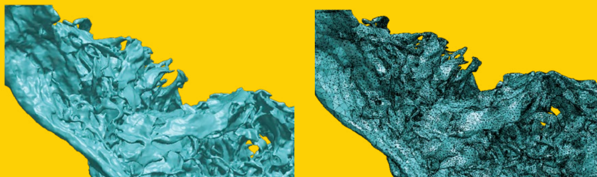
Simpleware software segmentation and FE mesh of birds nest showing level of detail
