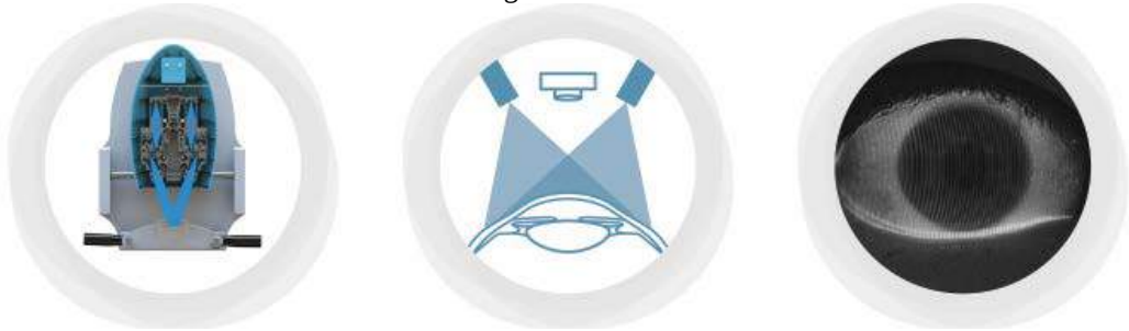
Figure 1 Eaglet-Eye ESP ocular topograph utilizing Fourier profilometry
