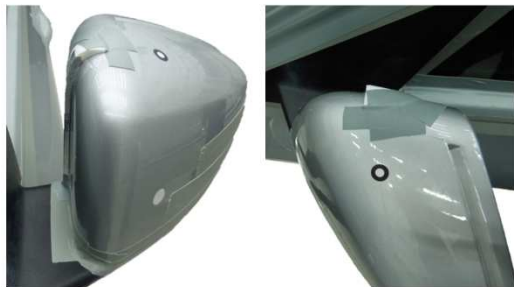
Figure 2: Side mirror modification (4 mm forward facing diffusor step)
