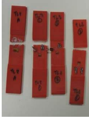
Figure 4: Post-test ABS specimens showing failure occurred in the gage length
