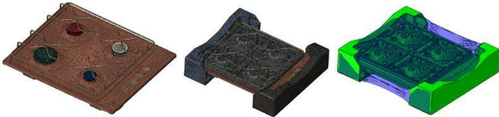
Figure 3 - the hob FEM model assembly is based on pre-meshed components db, the automatic mesh of the foam packaging and the automatic application of the thermal shrink film.
