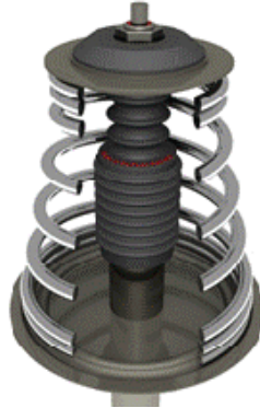
Figure 1. The jounce bumper is part of a vehicle's shock absorption system designed to absorb impact and dampen noise, vibration and harshness transformation option
