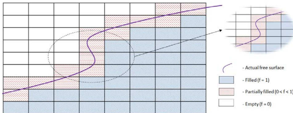
Figure 5. Volume of fluid method (VOF), f is volume fraction
