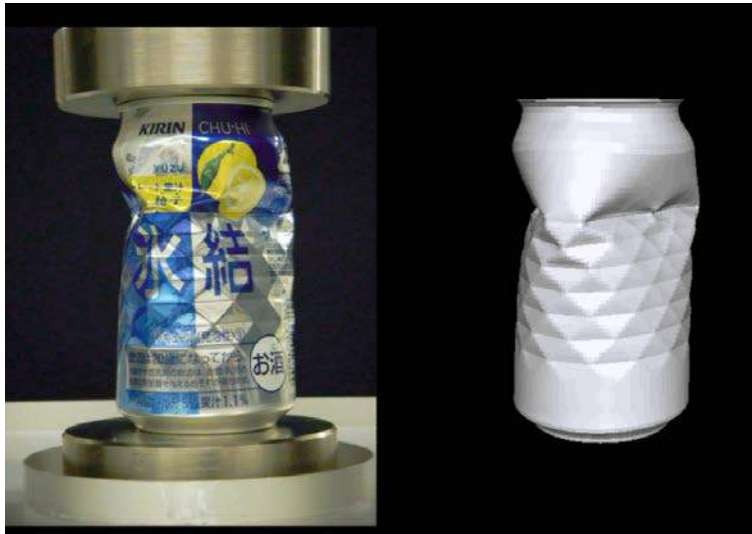
Figure 5. Beverage can under axial compression (Mihara and Kobayashi, 2008).
