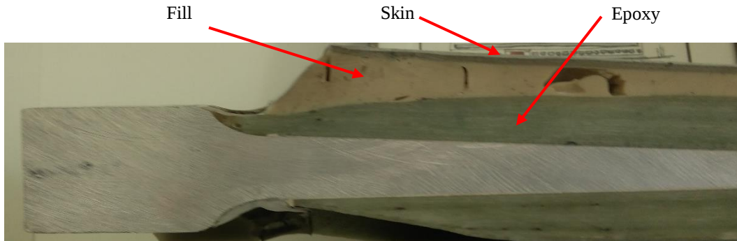
Figure 3. Connection of the aluring to the blade.
