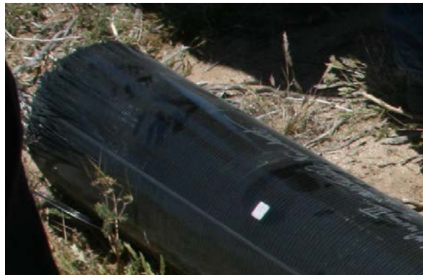
Figure 6. Flight motor static test: separated aft end of motor-case, fragment collected approximately 150 feet from test stand.
