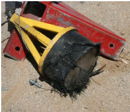
Figure 5. Flight motor static test: separated forward end of motor casing, fragment collected near test stand.
