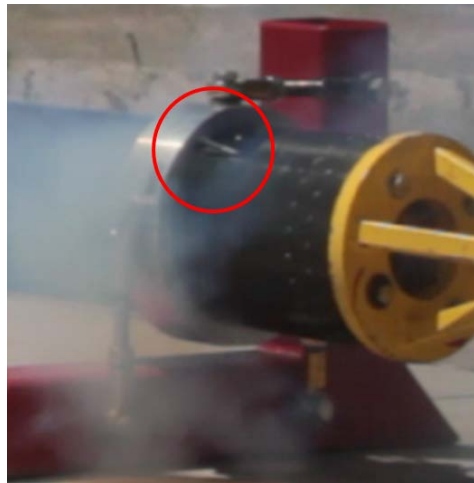
Figure 4. Fiber separation visible prior to catastrophic failure.
