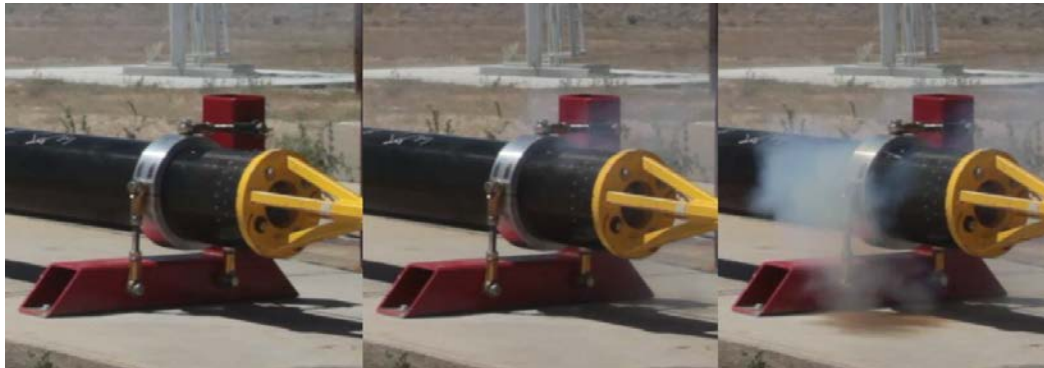
Figure 3. Frame-by-frame lead-up to motor separation.
