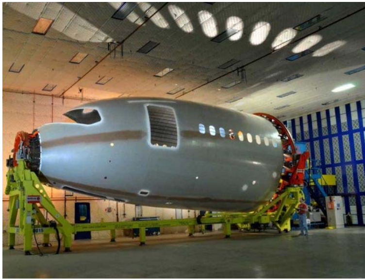
Figure 2. Boeing 787 Dreamliner forward fuselage manufactured by Spirit Aerosystems [3]
