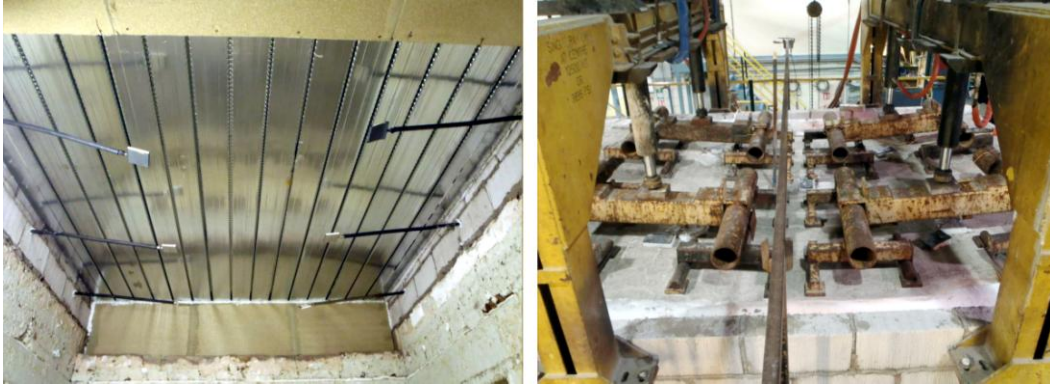
Figure 7 The exposed face of the test specimen prior to testing (left) and the unexposed face after 210 minutes of fire.
