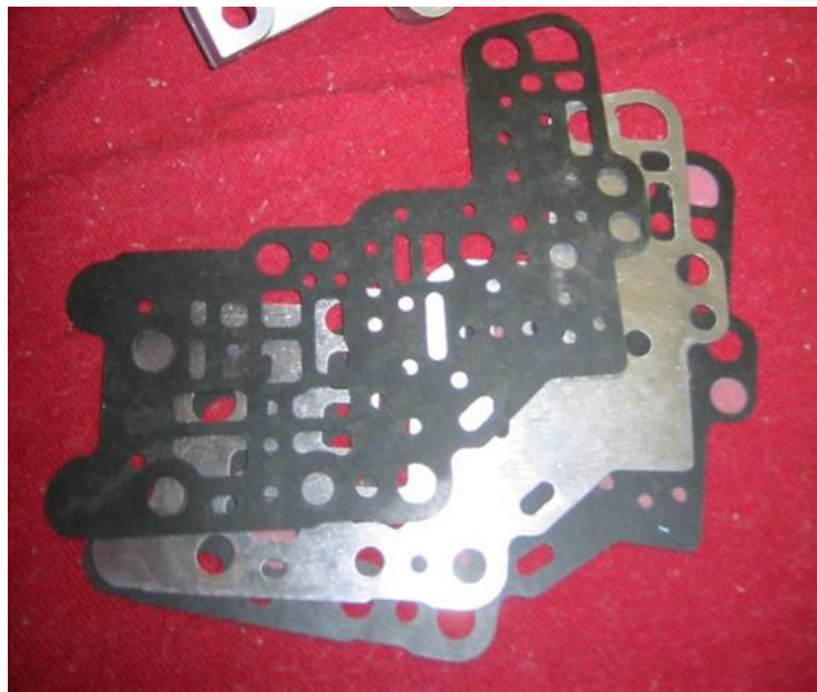
Figure 2. Steel plate -> low sealing potential
