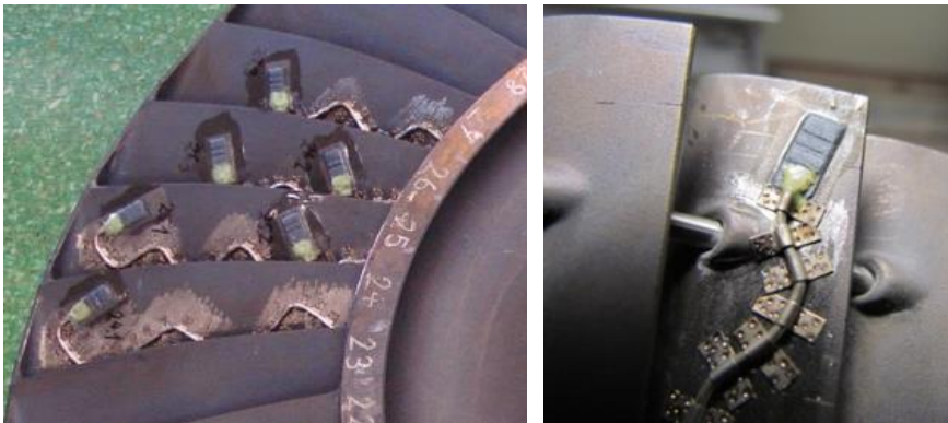
Figure 1. High-temperature strain gauge installation for blade vibration measurement
