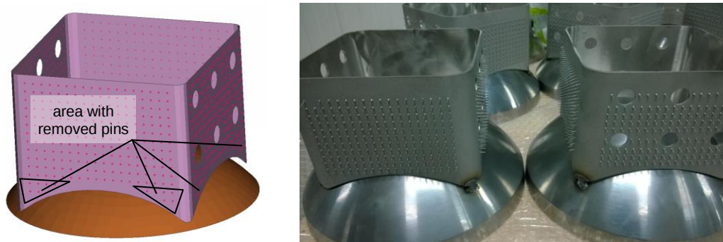
Figure 6: T-IGEL® pins at the FE- model and at the prototype parts
