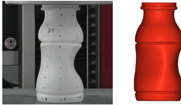
Figure 1. Top load test (left), simulation (right).
