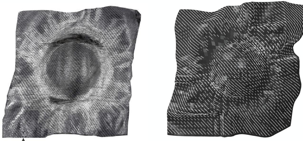
Figure 13. Predicted deformed shape of biaxial \pm 45 NCF (stitching reorientation is displayed with white-lines in FEM results).
