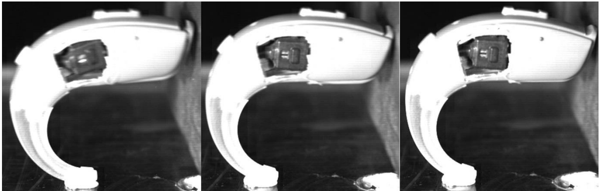
Figure 6. High speed video recording of impact. Left picture is 0.9 ms after impact. Middle picture is 0.1 ms after impact. Right picture is at impact.
