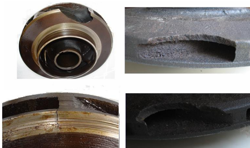
Figure 2. Fatigue crack and damage on an NK210/200 impeller.
