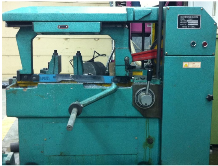
Figure 1. A reciprocated hacksaw machine.
