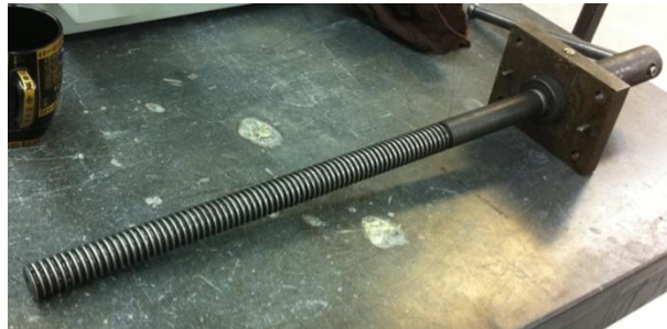
(b) Deformed power screw
