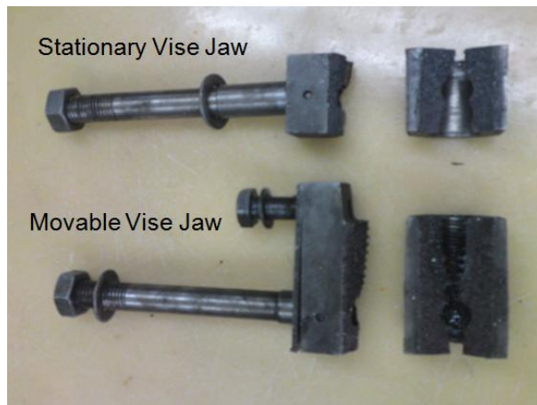
(a) Broken stationary and movable vise jaw holders
