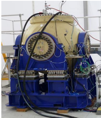
Figure 1 : Vessel for confined detonation experiments
