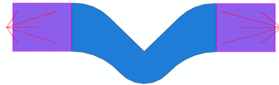
Figure 1. Kinematic coupling and symmetry boundary conditions of the Type C tear simulation for maximum and minimum gripping scenarios
