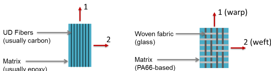
Figure 1: 'Classical' UD composite vs Vizilon™ TPC
